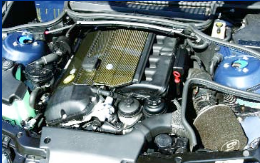
The TMS/Conforti air intake is the same used on the Grand-Am Cup 330i. Turner has dressed the engine compartment up with carbon fiber, and the fixed camber plates are visible through shock towers. A carbon-fiber gear lever handle is nice touch in the Performance Package interior.
