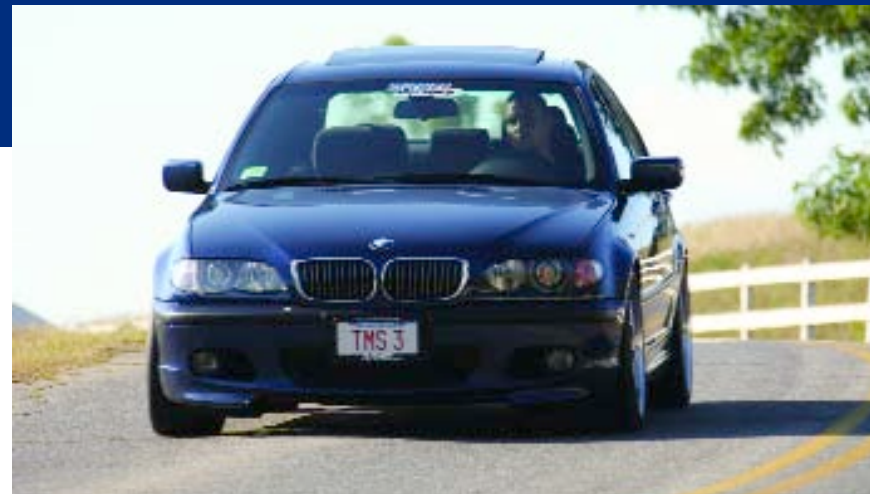
The TMS 330i puts out 252 horsepower and has handling that makes it an effective weekend warrior. The H&R RSS coil-over kit lowers the car and the BBS wheels really improve the sporty look; TMS rolled the inside of the fenders to avoid rubbing.
