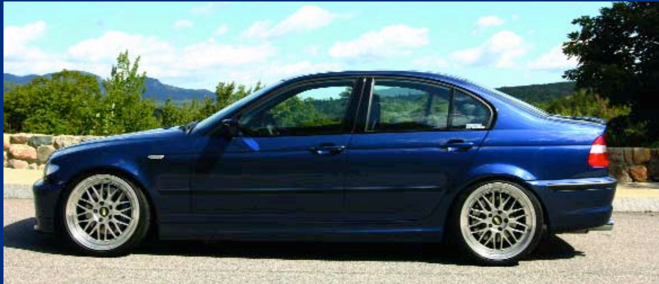
The TMS 330i puts out 252 horsepower and has handling that makes it an effective weekend warrior. The H&R RSS coil-over kit lowers the car and the BBS wheels really improve the sporty look; TMS rolled the inside of the fenders to avoid rubbing.
