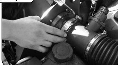
Tighten down 2 clamps that are used on the rubber adapter.
