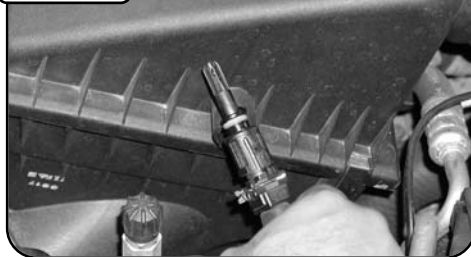
Remove temperature sensor from stock air box
