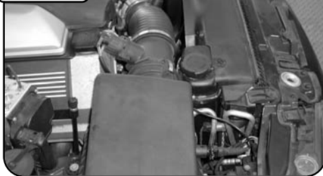
Remove bolt with 10mm socket or wrench and remove air box from engine.
