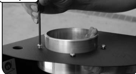
Assemble billet adapter to shield using 5 button head screws.
