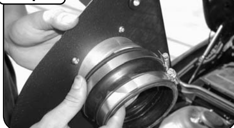
Slip on rubber adapter ( do not tighten).
