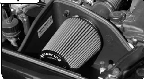
Make sure all hoses and clamps are tight and that all electrical components (if applicable) are secure. Check and retighten connections and filter after a few hours of operation.
