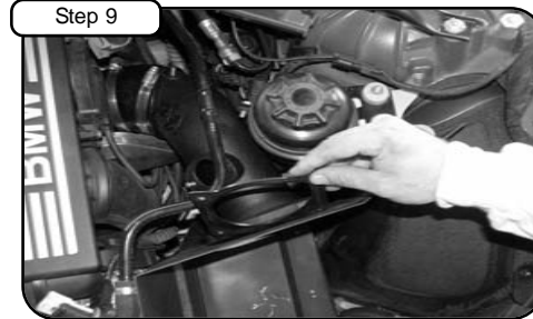
Install housing into vehicle. Place tube into coupler from step 8. With gasket provided, slide between tube and housing and wait for adapter install.
