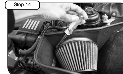
Install your high FLOW air filter. Tighten using 5/16" nut driver.
