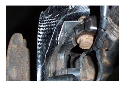
6. Reassemble rotor and caliper. Torque caliper bolts to: 110 Nm (81 ftlb)
